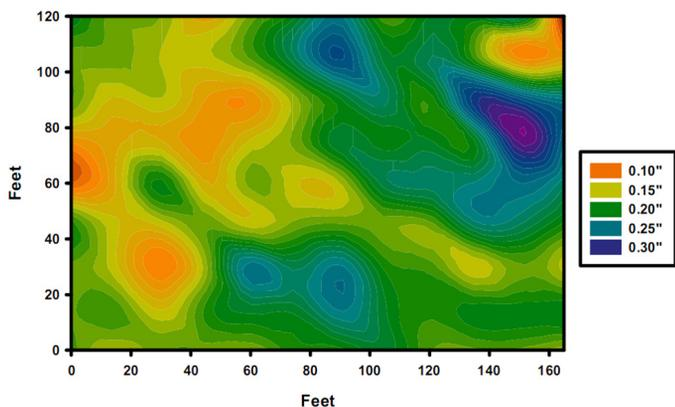
Figure 5. Map showing the distribution of water applied (in inches) on a fairway during a single irrigation event. Leaching may be insufficient to prevent the accumulation of salinity in areas that are chronically under watered as a result of non-uniform irrigation.
