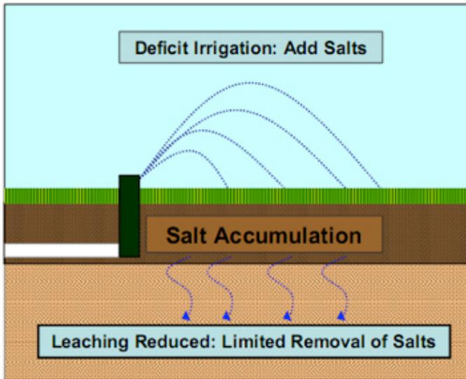
Figure 3. Deficit irrigation regimes develop when the amount of water received from irrigation and precipitation is insufficient to facilitate the level of leaching required to keep salinity levels at acceptable and stable levels in the root zone. Salts accumulate in the root zone and eventually reduce turf performance and damage soil structure.
