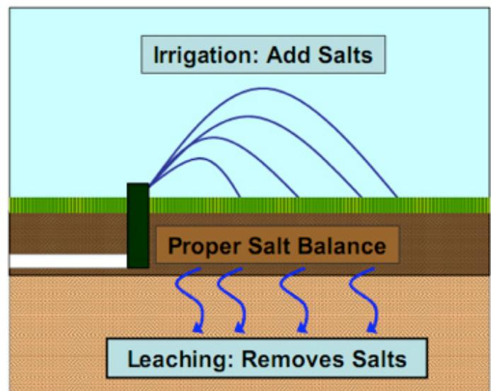
Figure 1. Water management regulates the salt balance of soils supporting turfgrass. Irrigation water continually adds salts to soil. Water in excess of evapotranspiration is required to facilitate deep percolation or leaching which removes excess salts, helping to maintain the proper salt balance in the root zone.
