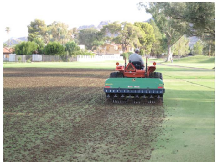
Figure 10. Tillage operations that create holes or slits in the surface soil can greatly improve infiltration and reduce the level of runoff. Deficit irrigation regimes can develop in areas prone to runoff, leading to poor turf quality and the accumulation of salts and sodium.
