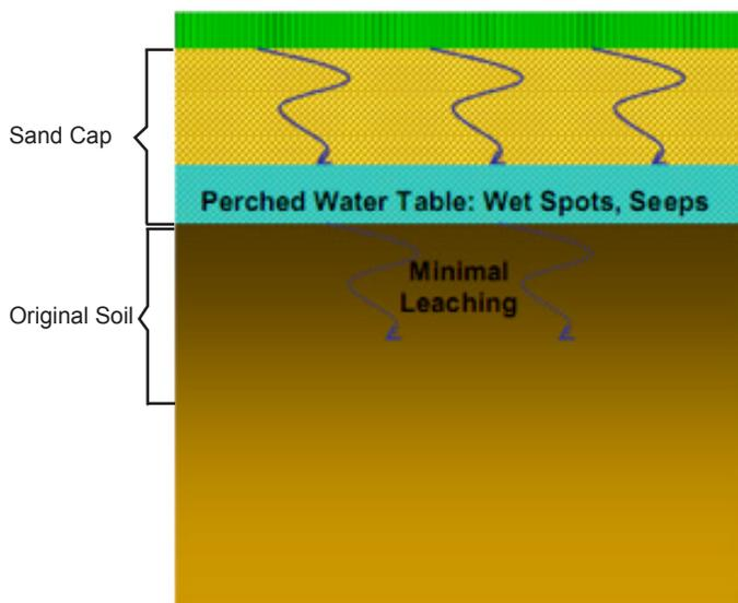
Figure 12. Capping poor infiltration soils with sand has been proposed as one means of improving infiltration rates. However, failure to improve the infiltration of the original soil surface (through chemical or mechanical means) prior to capping may result in the accumulation of water at the interface between the cap and the original soil surface. This accumulation of water is referred to as a perched water table and can lead to wet spots, seeps and the accumulation of salts in the sand cap.
