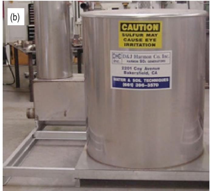
Figure 11. Applications of gypsum (a) can be used to increase the ratio of calcium to sodium in soils and thereby improve soil structure and infiltration. Lowering the pH of the irrigation water through the use of sulfur burners (b) or acid injection reduces the level of bicarbonate in the irrigation water which also improves the ratio of calcium to sodium in the soil.
