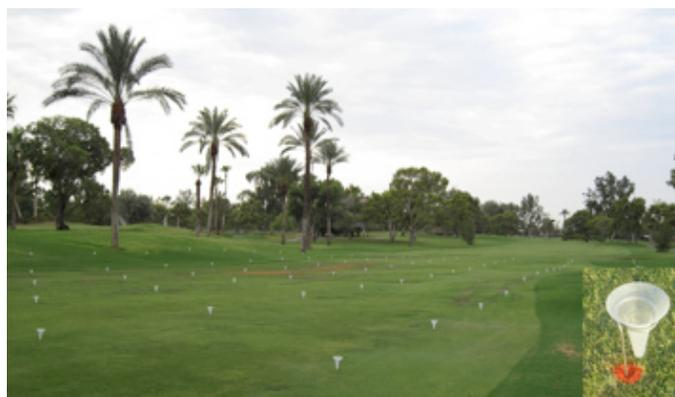
Figure 7. Catch cans (lower right) are graduated plastic containers used to quantify the amount of irrigation. Photo shows catch cans set out in an array to assess the amount and uniformity of an irrigation event.
