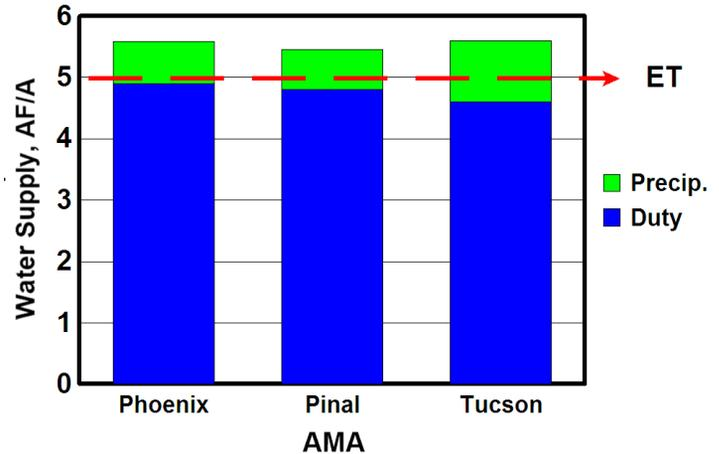
Figure 4. Potential water supply for turf irrigated with groundwater in the Phoenix, Pinal and Tucson Active Management Areas (AMA). Water supply consists of the water duty (amount of groundwater that can be used for irrigation; blue bar) and the average precipitation (green bar) for each AMA. Evapotranspiration (ET) of year round turf (red arrow) is similar in each AMA and exceeds the water duty.
