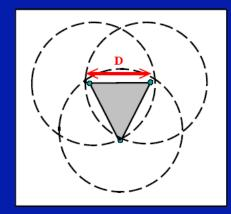
PR = (GPM \* 96.3)/[D<sup>2</sup> \*0.866]
