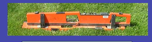
Non-Destructive Electromagnetic Induction Conductivity Meter
