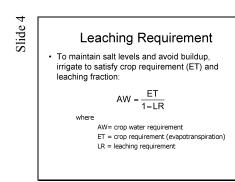
The amount of water we'd have to add to prevent salt buildup is calculated from the above equation.
