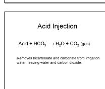
Levels of <u>carbonates</u>  $(CO_3^{2^-})$  and <u>bicarbonates</u>  $(HCO_3^{-})$  in irrigation water also should be monitored. These anions form insoluble compounds when they come into contact with calcium and magnesium. By effectively reducing calcium and magnesium levels in the soil, they increase the sodium adsorption ratio.
