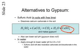
Acidifying agents all work by dissolving soil CaCO<sub>3</sub> (free lime), which produces gypsum. Sulfuric acid directly dissolves CaCO<sub>3</sub>. Any acid will do this. Sulfuric acid is the acid of choice because of relatively low cost and because it adds less salt to the soil than HCI (hydrochloric acid).
