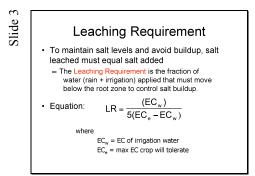
In addition to the irrigation water salinity ( $EC_w$ ), the leaching requirement also depends on the salinity tolerance of the crop being grown ( $EC_e$ ). The equation above can be used to estimate the leaching requirement.
