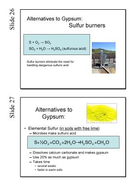
Sulfur burners convert elemental sulfur powder into sulfurous acid by combustion. They provide a safe way to inject acid into irrigation water.
